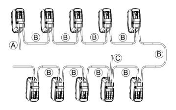
A: To connect the first TA-Slider 160/500 BACnet or Modbus of a daisy chain to the Bus.
