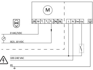
24 VAC/VDC operating only with safety transformer according to EN 61558-2-6.
