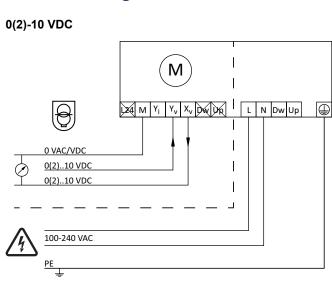
3-point I Μ MYi Yv Xv Dw DR L N DwUp  $\bigcirc$ θ 0 VAC/VDC I  $\langle \rangle$ 0(2)..10 VDC 100-240 VAC PE
