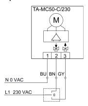
For 230V in 3-point control, the actuating direction can be changed by exchanging the **grey** and **brown** wires.
