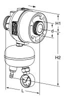
**DN 15-50 External threads** – Separate connections optional.
