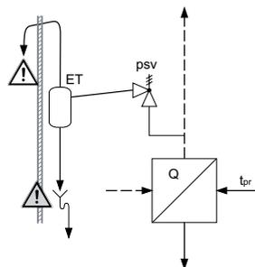
Expansion traps and dimensions for the supply and discharge according to national provisions.
