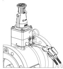
Connect IMI TA balancing instrument to the measuring points and measure  $\Delta \text{pL}.$
