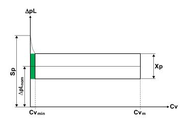
Sp = Sealing pressure, the increase of  $\Delta pL$  in psi when a  $\Delta p$  controller controls  $\Delta pL$  from  $Cv_{min}$  down to zero flow.
