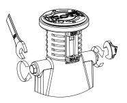
To vent the valve, open the topmost venting screw. **NOTE!** Max. 2 turns opening.
