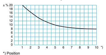
Try to avoid mounting taps and pumps, immediately before the valve.
