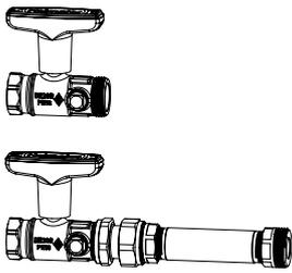
**Connection kit 4 with Globo ball valve DN 20, including spacer for heat meter in return**
