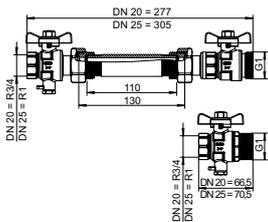
**Connection kit with ball valves, straight connection, including spacer for heat meter in return.**
