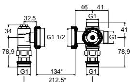
**Thermostatic mixing valve for radiant heating**
