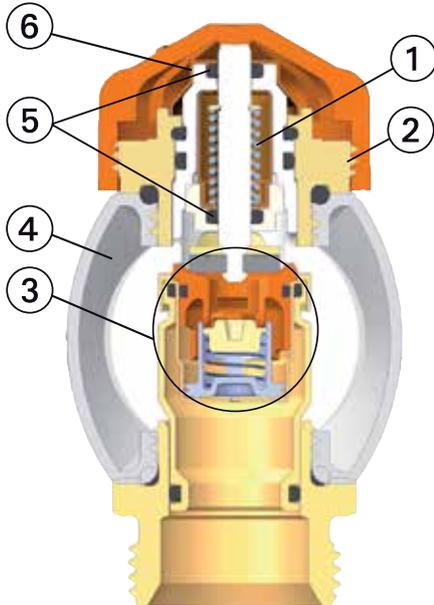
1. Strong return spring in combination with high locating force ensures that the valve does not slacken off over time
