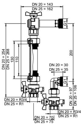
**Connection kit with ball valves, angle connection, including spacer for heat meter in return.**
