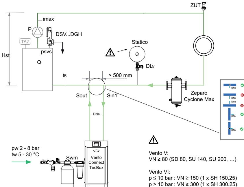
**Zeparo Cyclone Max** for the central separation of sludge.
