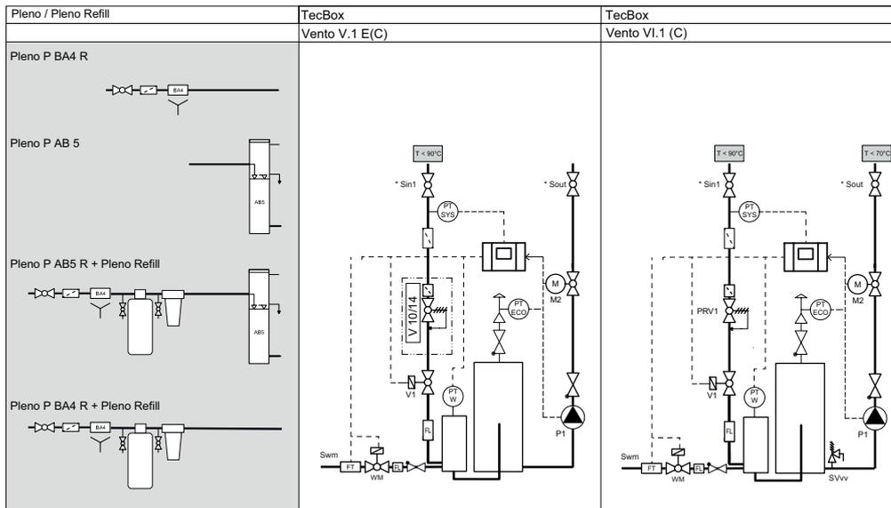
\* When connecting to rigid piping, it is essential to ensure that there is no axial, vertical or horizontal tension. The connections must not be loaded with any additional weights. Maximum tightening torques must be observed where specified. If no information on tightening torques is available, the state of the art for the respective connection must be observed. A flexible connection is preferred over rigid connection.
