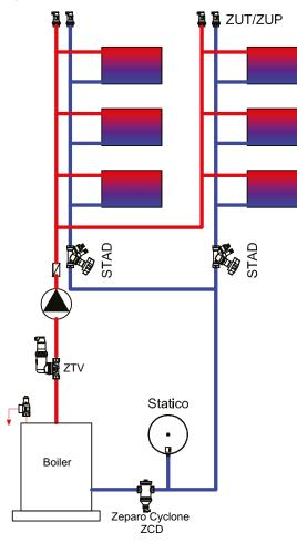
The Zeparo Cyclone dirt separator should be mounted either on the return in front of the unit to be protected or directly in front of the energy source.
