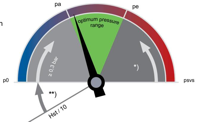
EN 12828, Solar, Cooling:  $\geq 0,2$  bar
