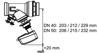
TA-Slider 750/1600 / TA-Slider 750/1600 Plus, Fail-Safe Plus
