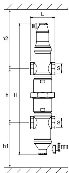
Suitable for the hydraulic decoupling of generators and consumer circuits, in combination with operational venting and de-sludging. To be installed between generator and consumer circuits. Integrated microbubble separation is only guaranteed if HB values are not exceeded. For optimal operation, the volumetric flow conditions as indicated below must be set between q1 and q2 (see case examples on page 5).
