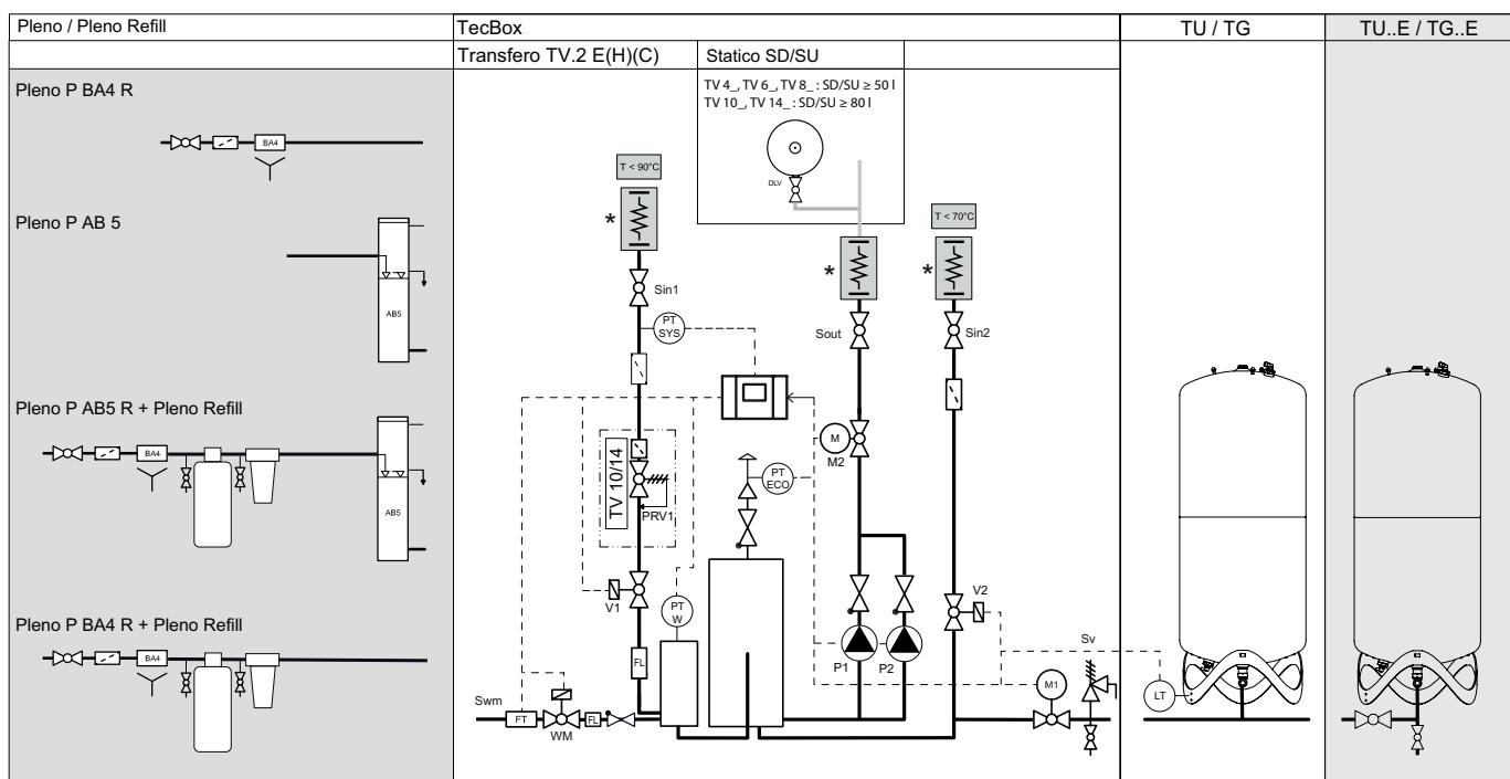
\* When connecting to rigid piping, it is essential to ensure that there is no axial, vertical or horizontal tension. The connections must not be loaded with any additional weights. Maximum tightening torques must be observed where specified. If tightening torques are not specified, the state of the art for the respective connection must be observed. **A flexible connection is preferable to a rigid connection.**
