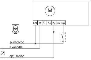
24 VAC/VDC operating only with safety transformer according to EN 61558-2-6.
