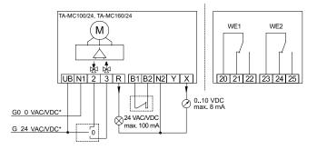
Automatic detection of broken control wire (for 2-10 V / 4-20 mA
