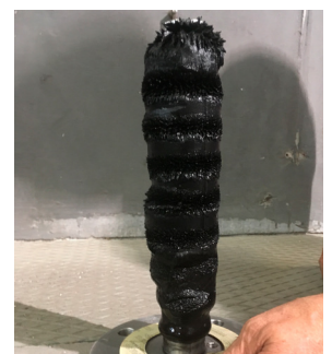
Ferro Cleaner magnet after 1 year of operation
