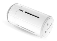
Halo-B is suitable for installation on all HEIMEIER thermostat valve bases and on valve radiators that have an M30x1.5 connection thread M30x1.5 on the upper part of the thermostat.
