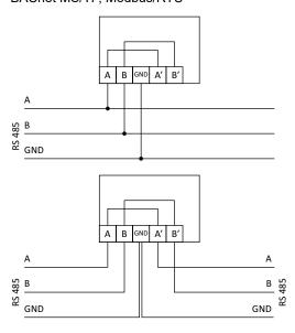
Note: A, B, A', B' and GND terminals are isolated from all other terminals.
