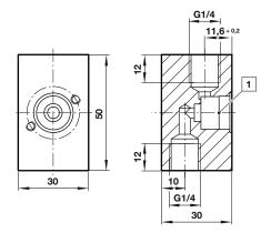
1 Interface geometry see Cartridge fitting D120.0010
