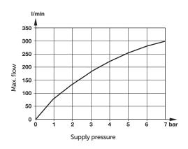
Flow vs. supply pressure curves are for informative purposes only and shall be used only for the pre-selection of the orifice size. Preliminary testing is recommended to take into account all application specific requirements and to select the most adequate orifice.
