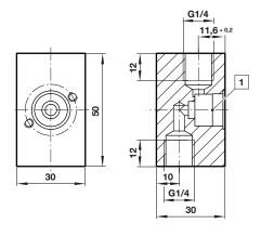
1 Interface geometry see Cartridge fitting D120.0010
