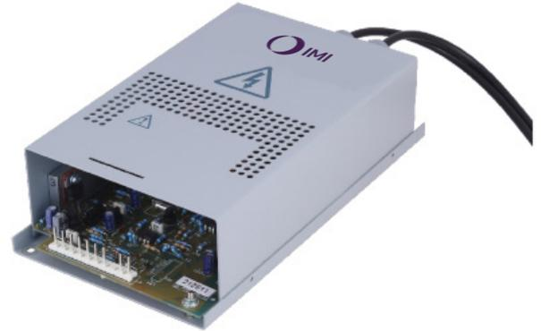
These power supplies are intended to electron multipliers, power microchannel plate and imaging detectors that are isolated by many kV from ground. They give 0 to +3.5 kV and can be floated on voltages up to  $\pm 2.5$  kV (HFxx2.5),  $\pm 10$  kV (HFxx010),  $\pm 20$  kV (HFxx020) &  $\pm 30$  kV (HFxx030). Contact factory for voltages other than 3.5kV.
