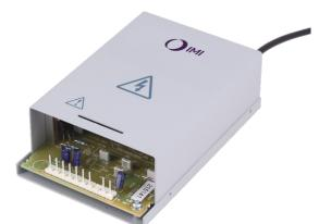
This range of precision high voltage modules has outputs that provide a low ripple, high stability source of high voltage for photomultiplier tubes, electron gun, nuclear and other applications. Control of the output voltage is by internal potentiometer or by an external 10 volt analogue control voltage. The units are pin compatible with the medium stability KS and 100watt HW ranges.
