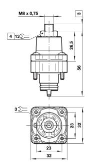
3 Adjustable from 0 to 7 mm Torque to 0,4/0,6 Nm maximum
